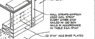
D13 SILL PLATE ANCHORS/ SLAB ON GRADE ANCHORS SILL PLATE AND STUD TO CONCRETE SLAB
